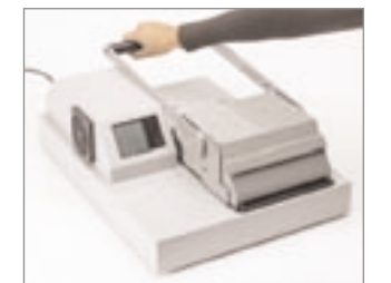
Close the flash machine and activate the flash (with most devices, the flash is automatically activated after the lid has been closed).
