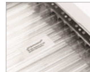
Place the printed vellum paper (right-reading) onto the glass surface of the flash machine.
