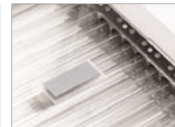
Place the flash text plate on top of the protective film (printing side facing downwards). Adjust the text plate with the help of the printed alignment frame. To ensure the printing is even when flashing, place a 2mm thick plastic or metal plate on top of the text plate.
